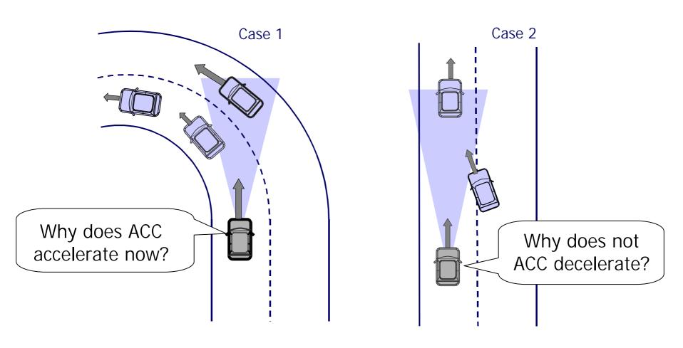
Fig. 1. Automation surprises caused by the Adaptive Cruise Control (ACC) system
