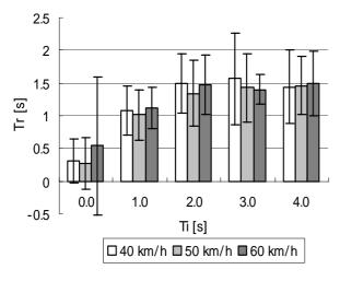
Fig.11. Response time by changing the speed of coming vehicle
